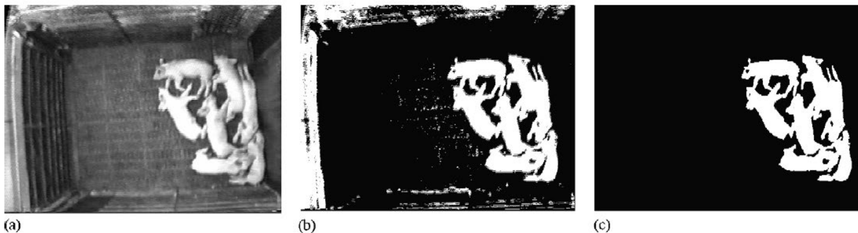
Fig. 6 – Example of system performance on image segmentation (under comfort condition). (a) Original gray-level image; (b) binary image after thresholding; (c) binary image after opening and blob filling.
